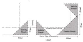
Figure 106.86-1 Visibility Triangles at Driveways and Intersections
